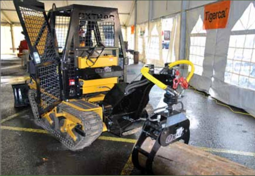
Tremzac's OxTrac hydrostatic skidder/forwarder attracted a lot of attention inside Triad's tent during this year's OLC. The manufacturer has just introduced a multi function remote controlled winch option for the versatile OxTrac. These functions include engage/disengage, throttle control, emergency stop, winch in/out.
