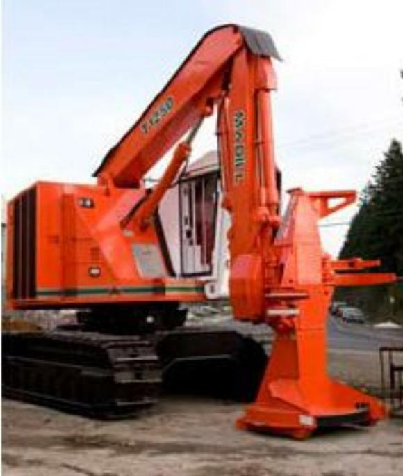
**Madill introduces its smallest leveling buncher**
